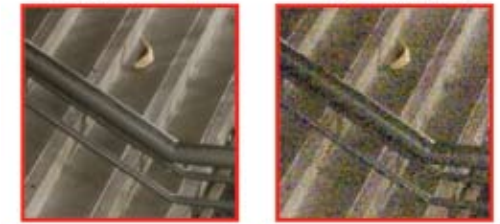
Digital cameras with adjustable ISO settings show similar tradeoffs to film performance. Higher ISOs provide greater light sensitivity, but with increased noise.
