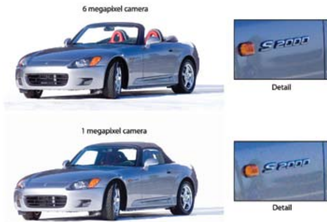
A resolution comparison between digital camera sensors. Lower resolution provides less image detail.
