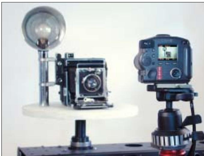
Figure 9.6: A simple object movie shooting setup: the object is mounted on a turntable, and the camera is on a tripod. (Photo by Scott Highton)
